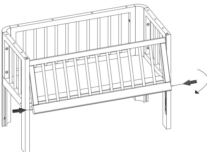
ENG: Push both of the pins in. While holding pins, move the side rail in the grooves
